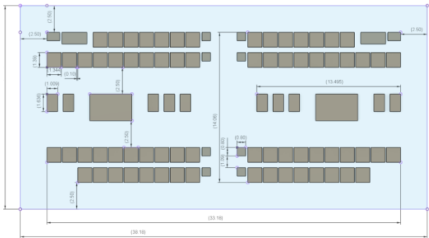
Figur 2 Situationstegning af batteriparkens interne layout
